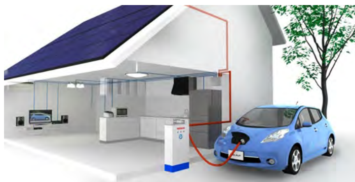
Figure 13 - Nissan vehicle-to-home system. Source: Nissan
