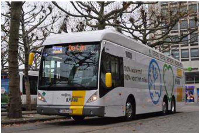
Figure 12: Fuel cell bus used by public transport operator De Lijn (Source: Van Hool)
