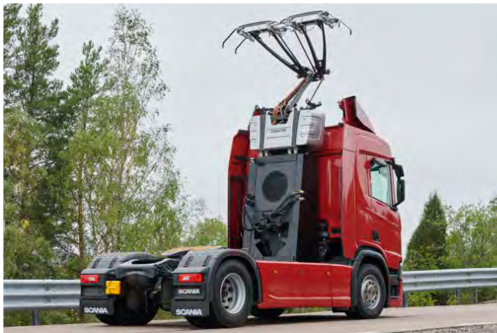
Figure 1: The type of SCANIA hybrid truck which connects to the Siemens' eHighway system.
