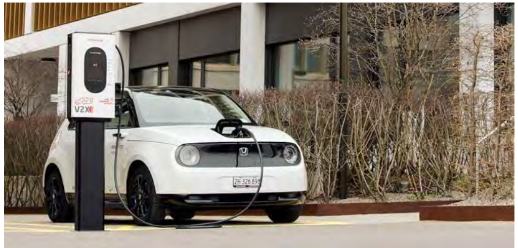
Figure 2: Bi-directional charging of a shared electric vehicle.
