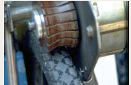
Friction roller drive on a solar bike from Russian solar bike pioneer Alexander Popolov, 1989.
