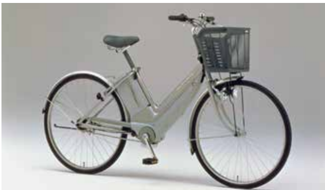
The Yamaha PAS pedelec, first sold in 1993 in Japan, was the first vehicle which, although it had a motorised assistance system, was legally classed as a bicycle because motor power was controlled so as to be proportional to muscle power.
