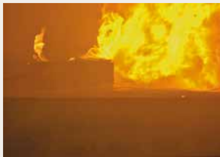
UNSAFE Eruptive conflagration shortly after a short circuit
