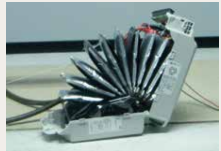
SAFE Cells are bulging due to overcharging and have broken their housing as a result, but have not ignited. Gases or fluids have not leaked.
