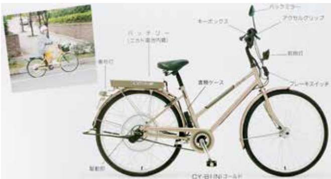
The San'yo electric bike, launched in 1989 in Japan. Because it was legally a motorbike despite its bicycle character, the user had to ride on the road and wear a motorbike helmet. These serious disadvantages were not acceptable to customers, and so there were very few buyers for this vehicle.
