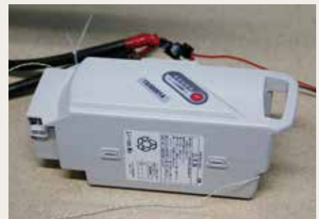
SAFE The BMS (Battery Management System) switches off quickly. In the second phase the electronics are bypassed. So the battery heats internally to over 100° C, but then cools again. Some fluid electrolyte has appeared, but no gases or other fluids.
