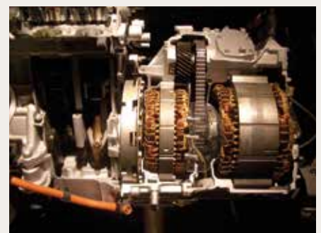
A role model for the pedelec – the principle of combining electric motor and IC engine, as solved in the Toyota Prius . For pedelecs it would work similarly, with the combination of electric and muscle power, for example in the futuristic prototypes from the company Nexxtdrive .
