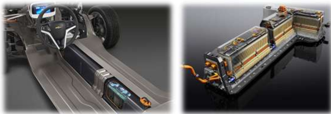
Fig 60: GM Chevrolet Volt (view of battery) 109
