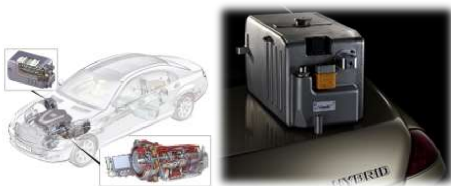
Fig 59: Daimler Mild- S 400 BlueHYBRID with Li-ion battery pack 108
