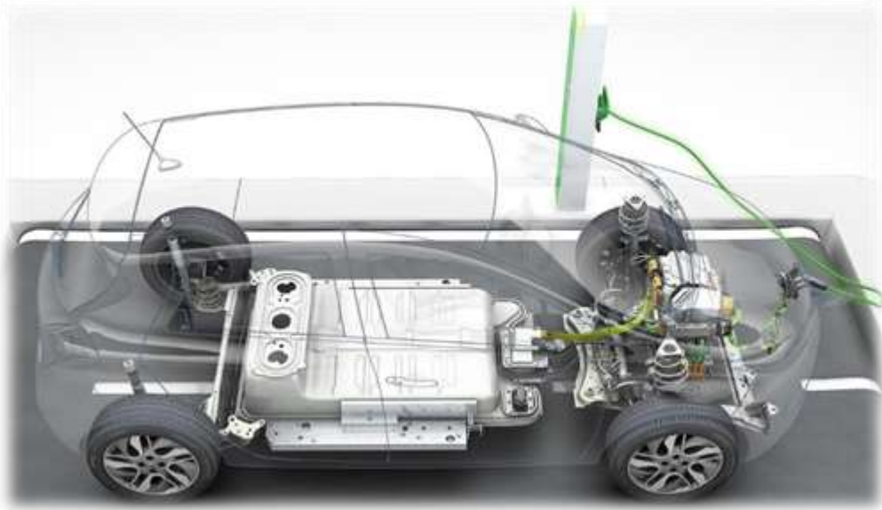
Fig 63: Battery module of Renault ZOE 112
