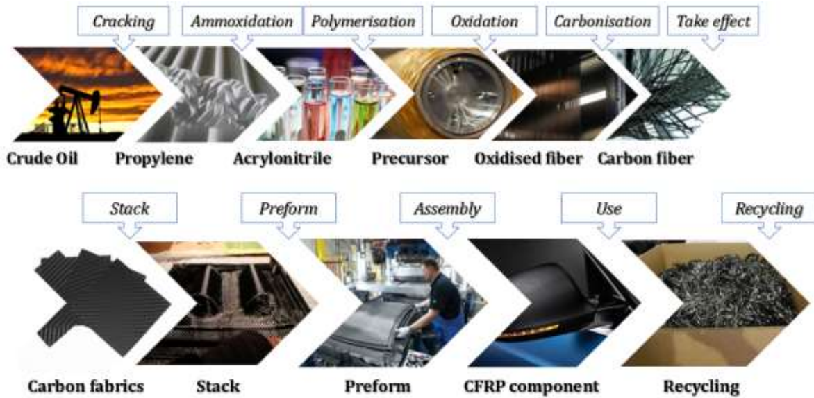
Fig 132: Carbon fiber production chain 192
