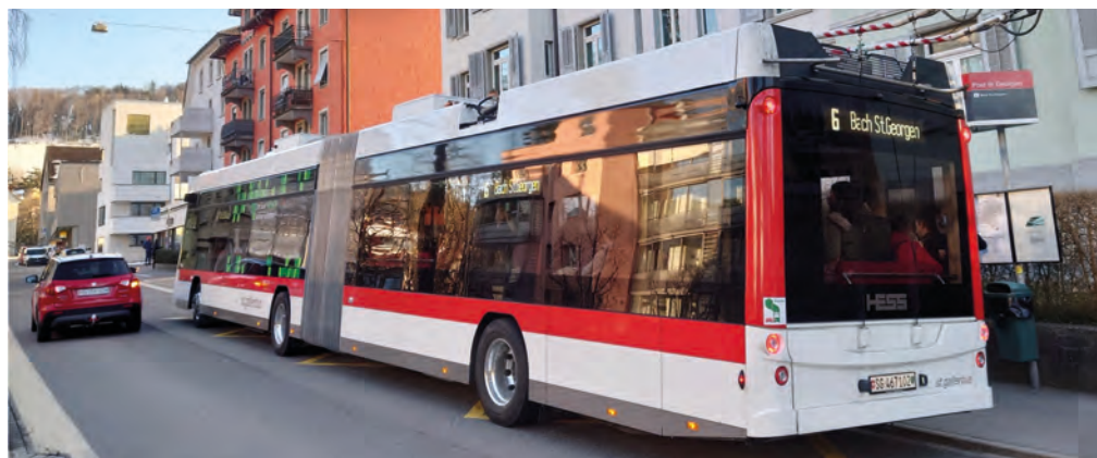
Figure 4: Hess lightTram 19 DC on VBSG line 6, in battery operation, at the station Post St. Georgen with lowered pantographs (Picture courtesy of EtschPat, via Wikimedia Commons).
