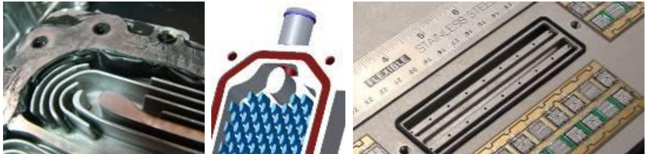
Figure 9 : Heat exchanger designs for power electronics : (left) Flat fins used in a Toyota Camry; (center) elliptical pin fin heat exchanger; (right) jet impingement cooling
