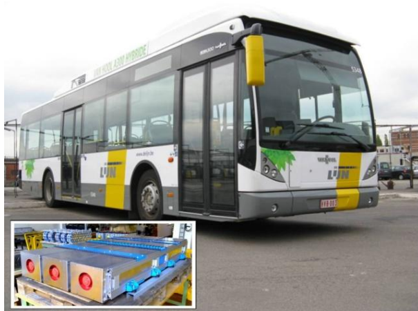
Figure 18: Brake-energy recovery on hybrid buses using ultracapacitors (inset) (Photo courtesy of Van Hool).
