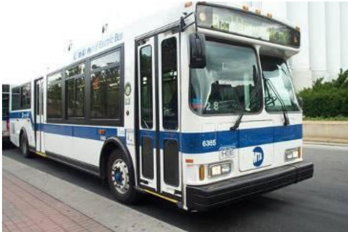
Figure 10 : Orion VII bus with BAE Systems HybriDrive hybrid propulsion system
