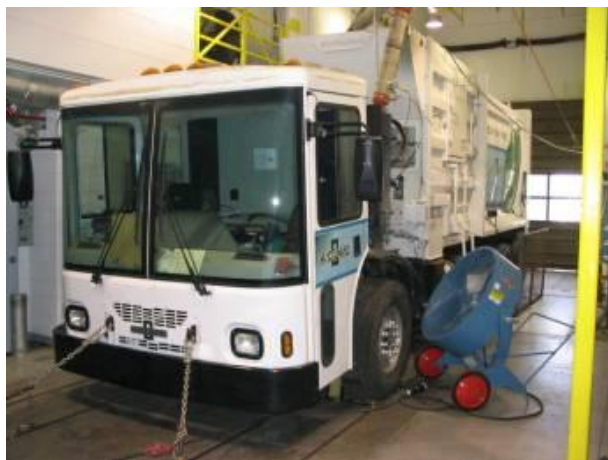
Figure 14: Oshkosh hybrid refuse hauler tested at NREL's ReFUEL Heavy Vehicle Chassis Dynamometer Facility
