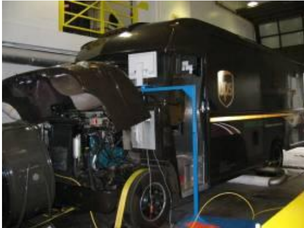
Figure 12 : Eaton hybrid system being tested at NREL’s Chassis Dynamometer Facility
