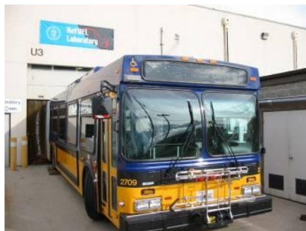
Figure 13: GM-Allison hybrid transit bus at the NREL ReFUEL Chassis Dynamometer Test Facility
