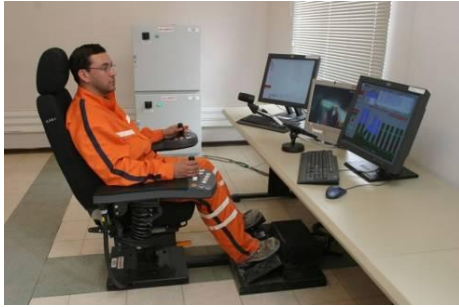
Figure 29: Automine control room
