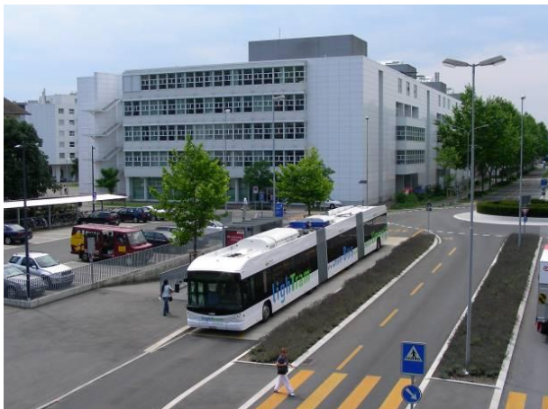
Figure 6 : lighTram@Hybrid with ultracapacitors (photo courtesy of HESS AG)
