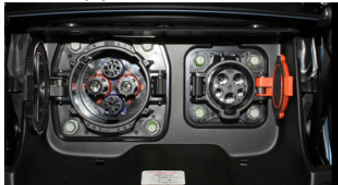
Figure 11: Nissan Leaf charging sockets: CHAdeMO (left) and ISO61196-2 Type 1 (right)
