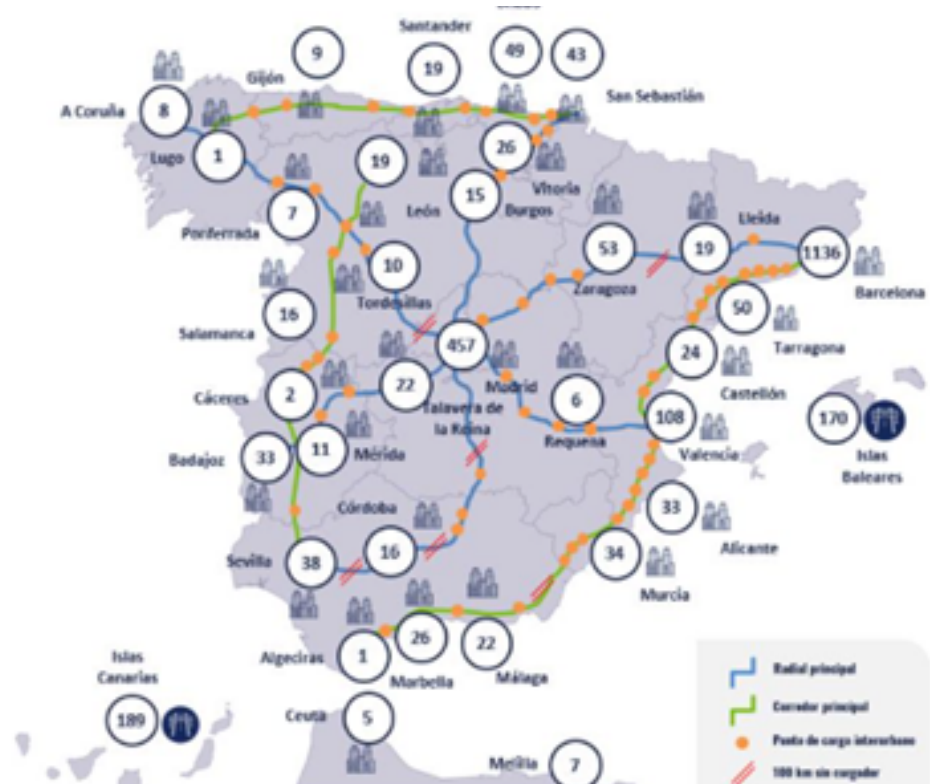
Figure 3: Recharging infrastructure deployed in the principal corridors, at the end of 2020 (Source: ANFAC)
