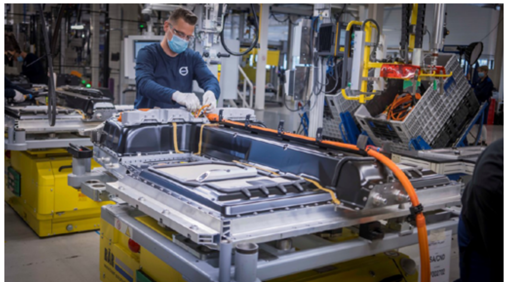
Figure 2: Battery assembly for electric vehicles at Volvo Cars' plant in Ghent, Belgium. (Source: Volvo Car Group)
