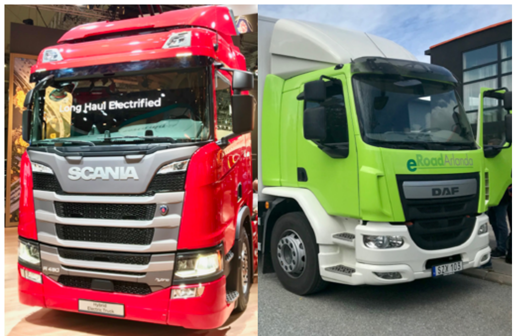
Figure 4: Scania plug-in hybrid trolley truck at the IAA Nfz fair 2018 (left) and electric converted DAF Truck tested in the eRoadArlanda (Sweden) project (right)
