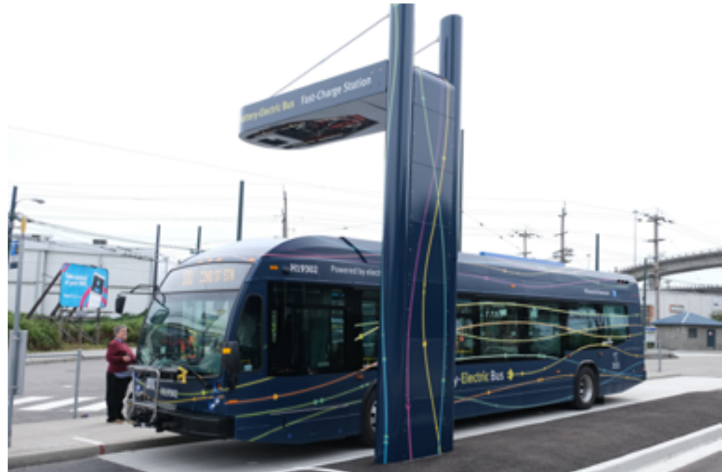
Figure 3: Overhead bus charger operated by TransLink in Vancouver, BC
