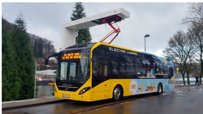
Figure 13: Volvo 7900 Electric Hybrid charging in Namur (Source: TEC Group)
