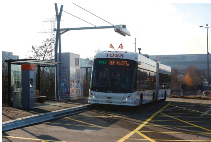
Figure 4: A TOSA bus approaches a bus stop equipped with a charging station (Source: www.ge.ch )
