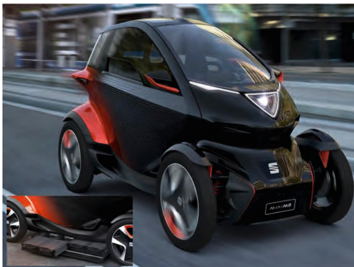
Figure 2: The Seat concept micro car with manual swappable batteries which MINIMO designed to be used in dockless sharing systems (Source: Seat)
