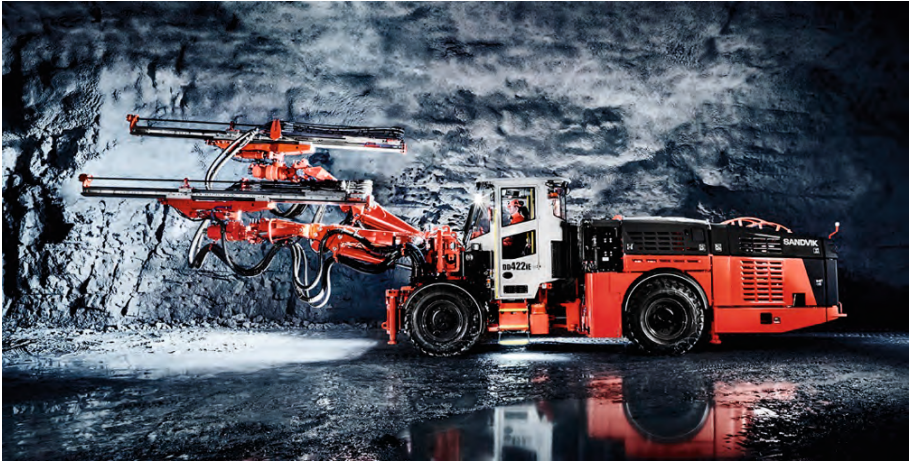
Figure 8: Sandvik DD422iE is part of the all-electric fleet at Borden Lake (Source: Sandvik)
