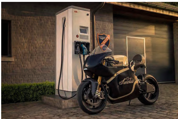
Figure 6: Saroléa SP7 electric race bike with DC quick-charge capabilities (Source: Saroléa)
