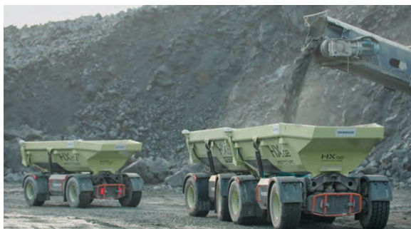
Figure 4: Volvo HX02, a battery electric, autonomous dump truck with 15 metric tons load capacity
