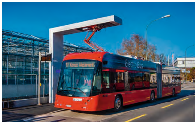
Figure 5: TOSA variant with a pantographic charging system (Source: www.bernmobil.ch )
