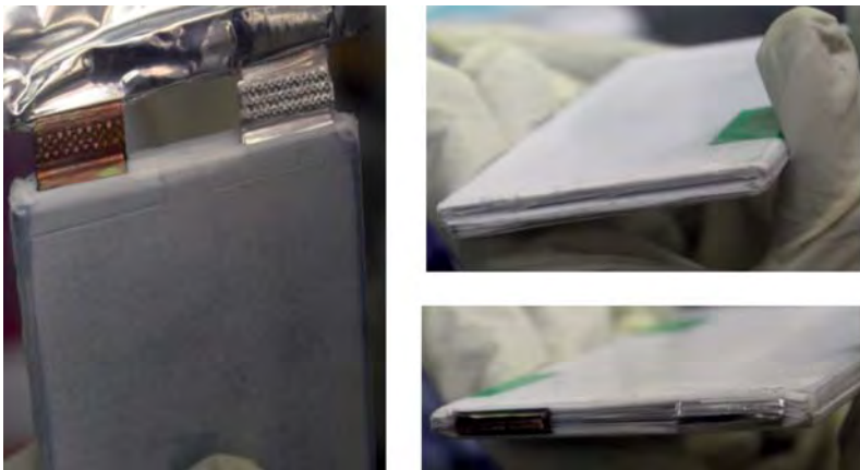
Figure 1: Images of an 11 Ah capacity pouch cell undergoing teardown and failure analysis (Source: private)
