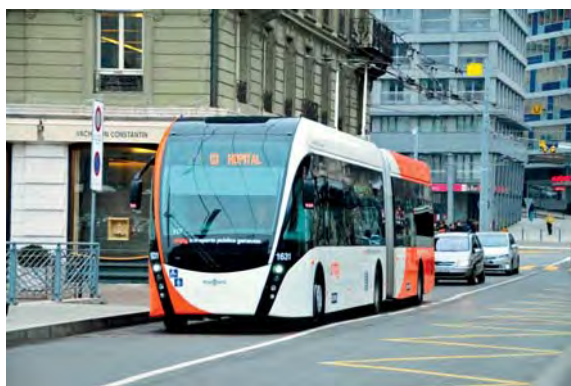
Figure 3: EquiCity Articulated Trolleybus with battery APU for TPG Geneva (Source: Van Hool)
