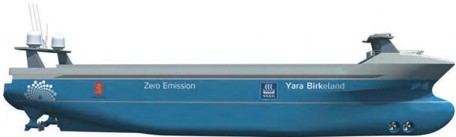
Figure 8: The first fully electric and autonomous container ship in the World (Source: https://www.km.kongsberg.com/ks/web/nokbg0240.nsf/AllWeb/4B8113B707A50A4FC125811D00407045?OpenDocument )
