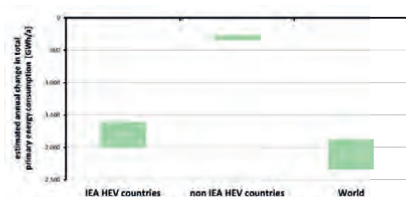
Figure 14: Estimated range of change in cumulated primary energy consumption of EVs substituting ICE globally in 2015
