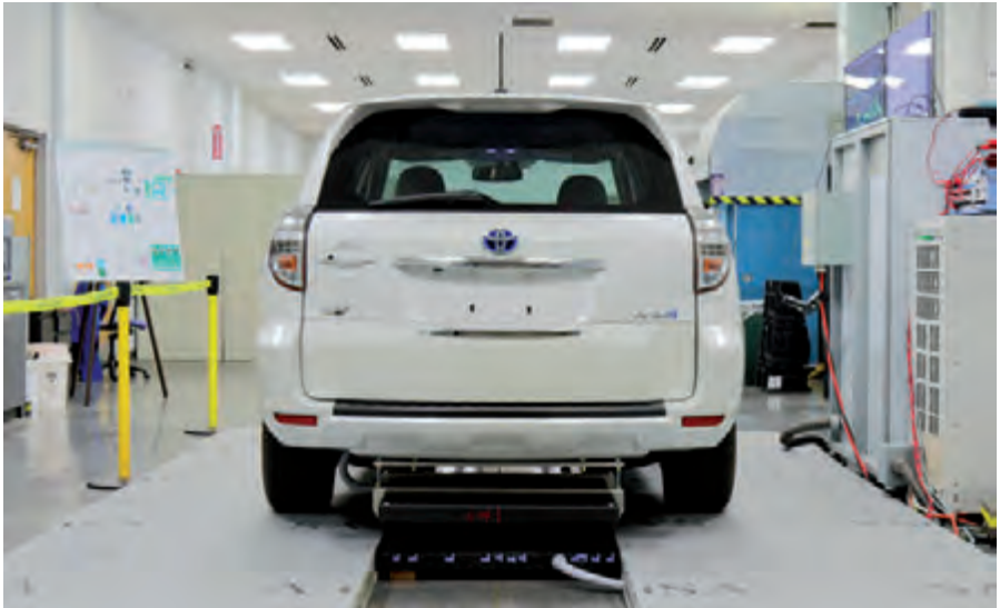
Figure 2: Demonstration of static wireless charging of a Toyota RAV4 with Oak Ridge's wireless charging system (Source: ORNL)
