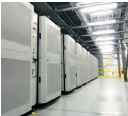
Figure 10: Automated cell finishing lines improve battery cell cycle life and performance (Source: PEC)
