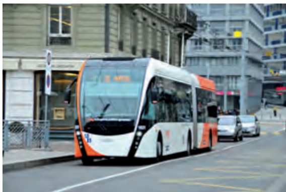
Figure 4: EquiCity Articulated Trolleybus with battery APU for TPG Geneva (Source: Van Hool)
