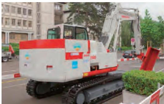
Figure 7: SUNCAR's low-noise and energy-efficient e-digger (Photo: NTB)
