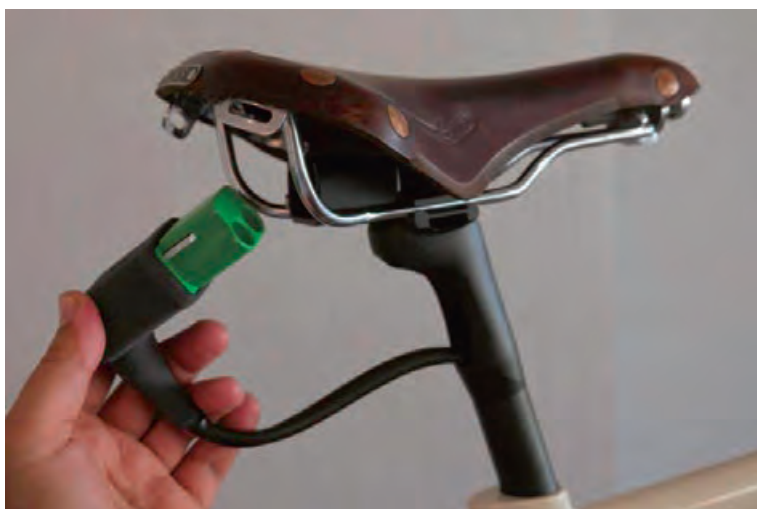
Figure 4: The Charge & Lock cable sample embedded in a bicycle saddle and its seat post. If not in use it is almost invisible and out of the way.
