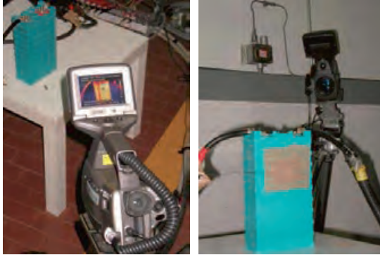
Figure 3: Second-life abuse testing equipment for aged Li-ion modules (Image courtesy of ENEA)
