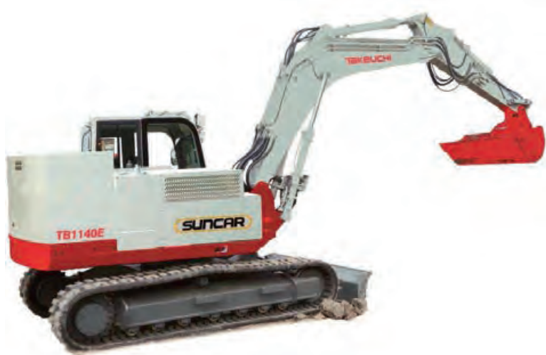
Figure 3: The suncar excavator with 15,400 kg weight and gravel force of 98,700 N is another application for the electric drive
