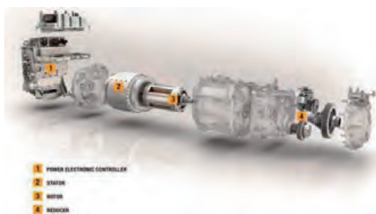
Figure 5: Renault improved the performance of their EV 'ZOE' by improvement of the power electronic and electrical architecture 11
