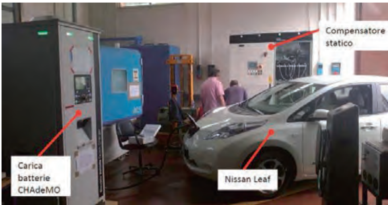
Figure 5: Integrated testing station for fast charger characterization and static compensator for evaluating the impact on the electricity grid (Image courtesy of ENEA)
