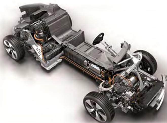
Figure 1: BMW i8 drivetrain (image courtesy of BMW 6 )
