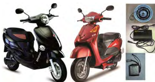
Figure 5: 2W EV Photon and Optima from HeroEco, on the left hand side, and YO-EXL 2W EV from Electrotherm with its motor, charger and BMS, on the right hand side.
