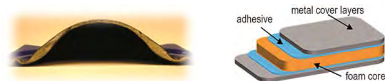
Figure 4: Material "Cimera" (left), schematic drawing (right) (image courtesy of 4a manufacturing)
