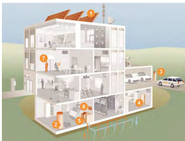
Figure 1: Elements of GridSense: 1 Photovoltaic system | 2 Boiler | 3 Charging station for electric vehicles | 4 House battery | 5 Heat pump | 6 Gateway | 7 Control app/Web (Photo: Alpiq)
