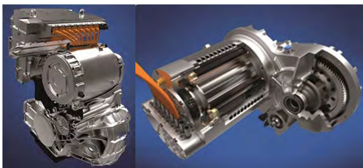
Figure 8: Hybrid (left) and full electric (right) powertrain with SR-motor (Source: Punch Powertrain)
