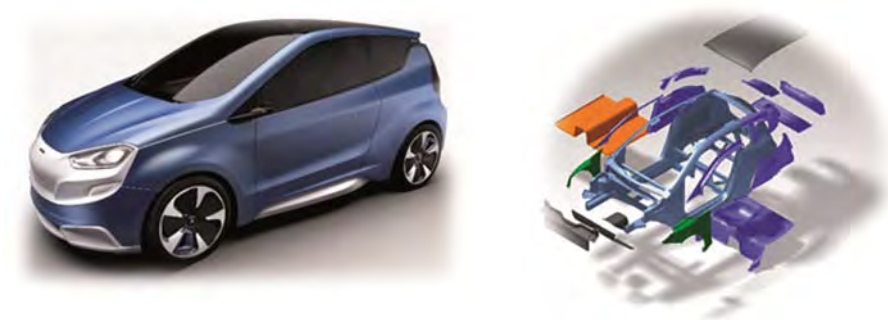
Figure 8: CULT, vehicle (left) and explosion view (right) (image courtesy of Magna)
