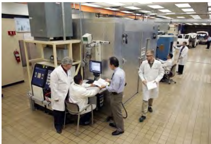
Fig. 10.1 Accelerated testing of Li-ion batteries. (Image courtesy of NREL [National Renewable Energy Laboratory])
