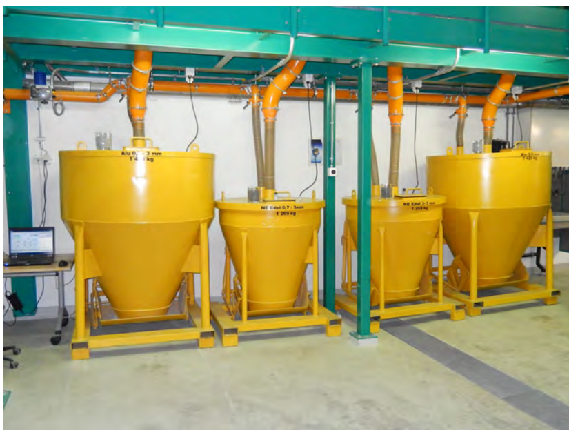
Fig. 8.3 Separation of metals from ash and slag at the pilot facility of KEZO/MVA in Hinwil, Switzerland.
