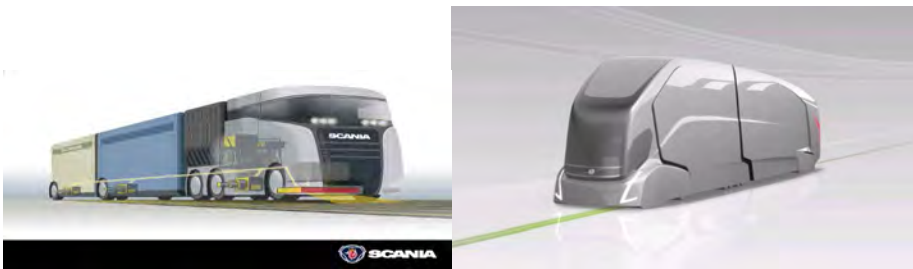
Fig. 25.1 Electric road systems with inductive (wireless) transmission, as under development by Scania and Bombardier (left), and with conductive transmission as under development by Volvo and Alstom (right). (Images courtesy of Scania and Volvo/Alstom)
