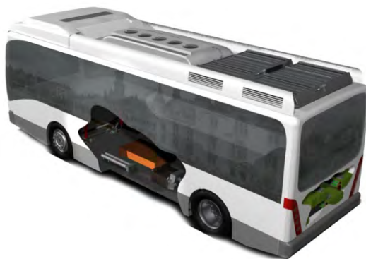
Fig. 14.2 Full electric bus with contactless inductive power transfer. (Photo courtesy of Van Hool.)
