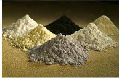
Fig. 30.2 The use of rare earth elements for use in batteries has increased dramatically over the past years. Clockwise from top center: praseodymium, cerium, lanthanum, neodymium, samarium, and gadolinium. (Photo courtesy of U.S. Department of Agriculture.)
