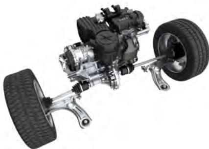
Fig. 13.2 AVL e-fusion modular system for hybrid powertrains. (Photo courtesy of AVL List GmbH.)
