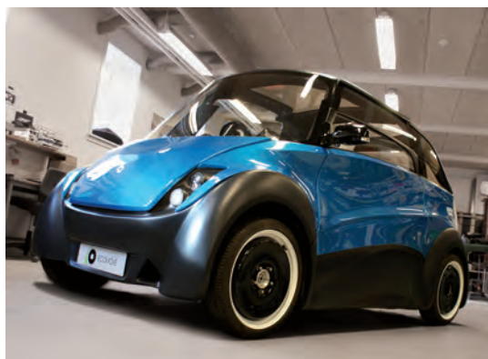
Fig. 16.2 The QBEAK EV from ECOMove has large cabin space despite outer dimensions of 3 meters by 1.75 meters, and can have a range of up to 300 km, based on the number of battery modules installed. (Photo courtesy of ECOMove.)
