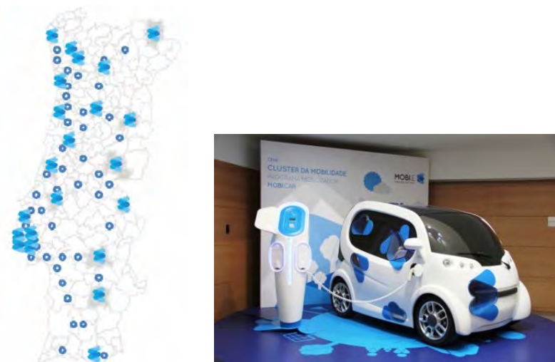
Fig. 23.2 MOBI.E vehicle electrification project includes installing charging stations in 25 municipalities and along main highways in its pilot phase as well as developing an 80-km range battery-electric vehicle, Mobicar, primarily aimed at the export market. (Source: MOBI.E)
