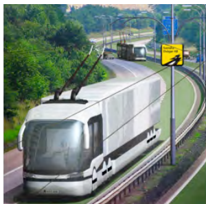
Fig. 25.1 A concept picture from the Swedish company Svenska Elvägar that run one of three projects that the Swedish Energy Agency is financing about electric roads. The pantograph system connects to the overhead power line at vehicle speeds up to more than 80 km per hour. (Photo courtesy of Svenska Elvägar.)
