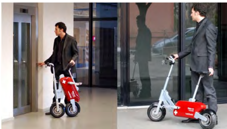
Fig. 5.2 Full production of the Voltitude begins in 2012. This e-bike folds for easy storage and weighs around 50 pounds (23 kg). It is equipped with a 250-watt integrated motor powered by a 36-volt lithium-ion battery. (Photo courtesy of www.veloland.ch .)
