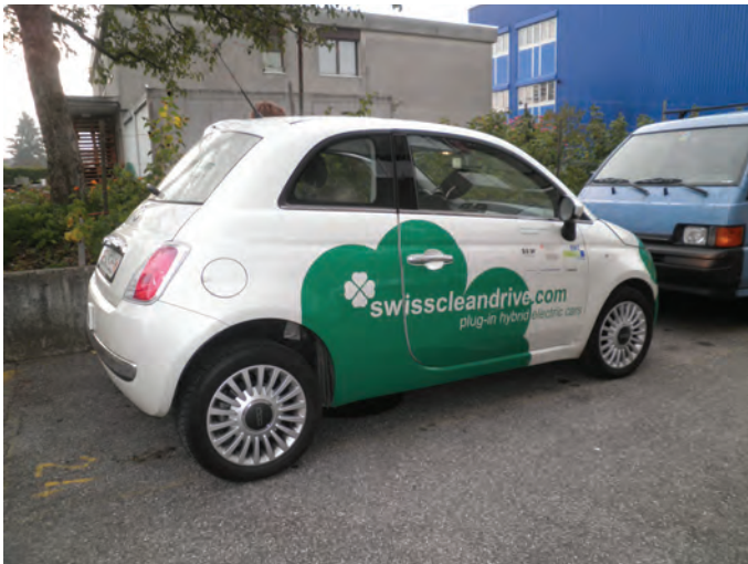
Fig. 26.2 SwissCleanDrive Fiat 500 converted to a plug-in hybrid car. (Photo: Solarcenter Muntwyler.)
