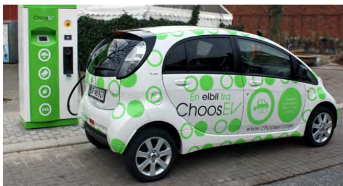
Fig. 16.4 ChoosEV test vehicle and quick charge station (using the CHAdeMO protocol) developed in cooperation with Siemens. (Photo courtesy of ChoosEV.)
