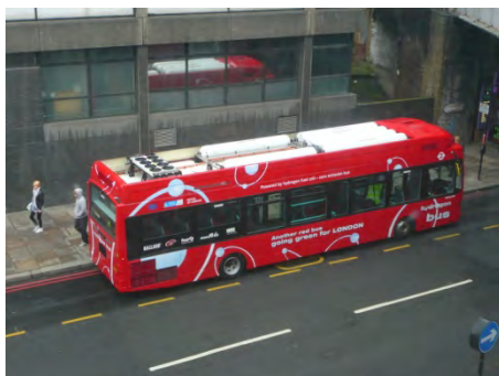
Fig. 15.9 Hydrogen fuel cell buses for London. (Photo courtesy of Bluways.)
