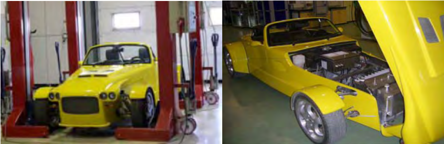
Fig. 28.1 TÜBITAK MRC Energy Institute sodium borohydride fuel cell vehicle prototype. (Photo courtesy of TÜBITAK MRC Energy Institute.)
