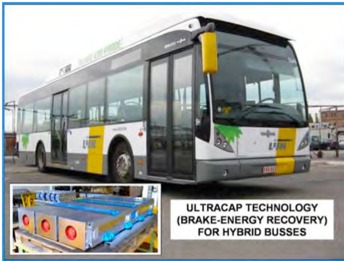
Fig. 15.3 Brake-energy recovery on hybrid buses using ultracapacitors (inset). (Photo courtesy of Van Hool).
