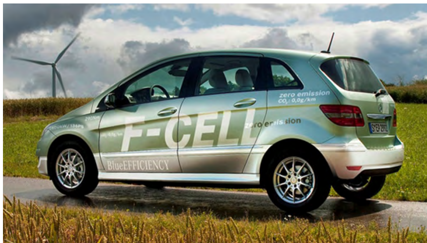
Fig. 8.1 Mercedes Benz B-Class (2009). Motor output (continuous/peak): 70 kW/100 kW. 80 kW PEM fuel cell system and lithium-ion battery with an output of 24 kW/30 kW (continuous/peak) and a capacity of 1.4 kWh to boost power and recover braking energy. Fuel: hydrogen at 700 bars. (Source: www.mercedes-benz.de .)
