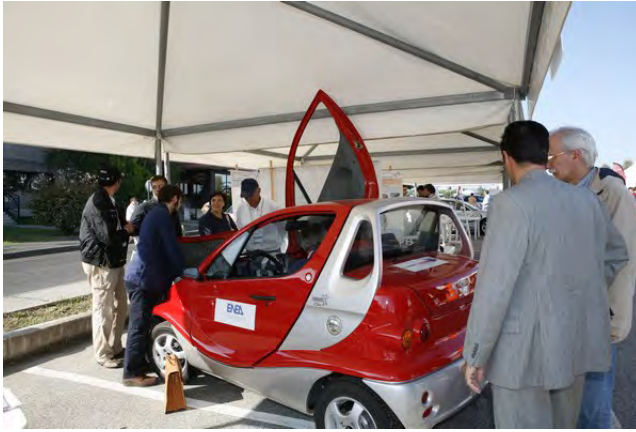
Fig. 20.2 Light electric City-car prototype with supercapacitors, developed by ENEA. (Photo supplied by ENEA)
