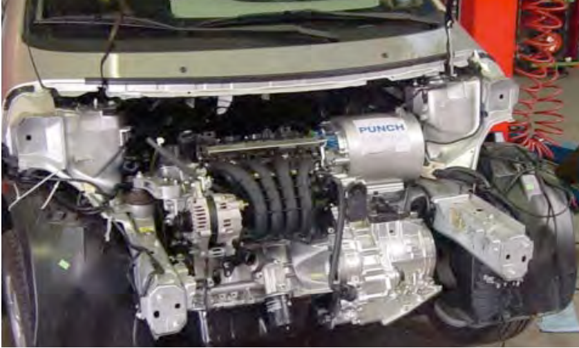
Fig. 15.9 Powertrain being integrated into a demonstrator vehicle. (Photo courtesy of Punch Powertrain.)
