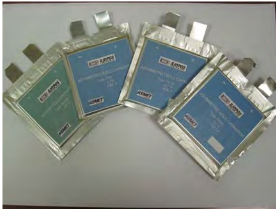
Fig. 20.1 ILHYPOS asymmetric and hybrid prototype cells with ionic liquid in the electrolyte. (Photo supplied by ENEA.)
