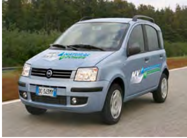
Fig. 20.5 Fiat Hyper Panda that uses hydrogen-natural gas blends. (Photo supplied by ENEA.)
