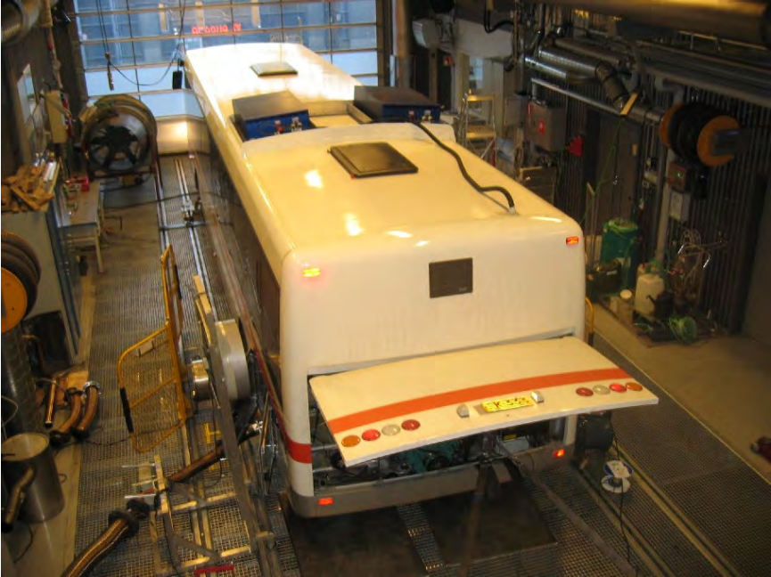
Fig. 11.1 A prototype hybrid bus being tested in VTT's chassis dynamometer facility. (Photo supplied by VTT.)
