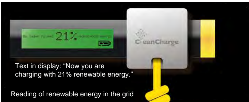
Fig. 17.5 CleanCharge equipment displaying the actual rate of electricity from wind power in the grid. (Photo courtesy of CleanCharge.)
