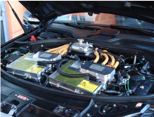
Fig. 14.2 Under the hood of the lithium-ion battery equipped HySUV from Magna Steyr. (Photo: M. van Walwijk.)
