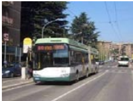
Fig. 12.4 As part of a policy for cleaner urban air, in March 2005 the Italian capital city of Rome re-installed a trolley bus line. The new trolley buses have onboard batteries powerful enough to allow as much as 3 km of unwired operation through the city centre. (Photo courtesy TrolleyMotion.)
