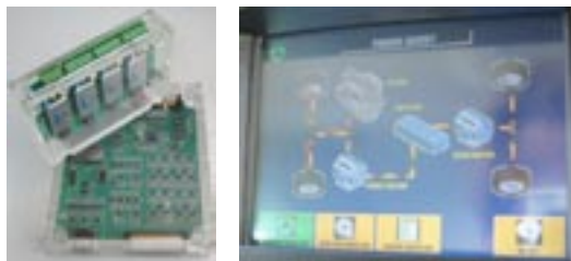
Fig. 23.2 HEV electronic control unit (HECU) and user interface developed by TÜBİTAK MRC Energy Institute. (Photos supplied by TÜBİTAK MRC.)
