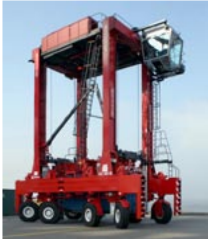
Fig. 17.1 Cargotec's Kalmar business unit presented the world's first straddle carrier equipped with a hybrid drive system in June 2008. (Photo supplied by the Helsinki University of Technology.)
