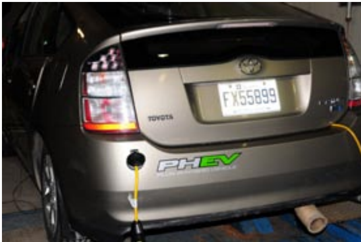
Fig. 11.1 Plug-in hybrid electric vehicle conversion in Environment Canada's test laboratory. (Photo: S. Furino.)
