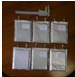
Fig. 19.1 ILHYPOS symmetric carbon/carbon prototype cells using ionic liquid in the electrolyte. (Photo supplied by ENEA.)
