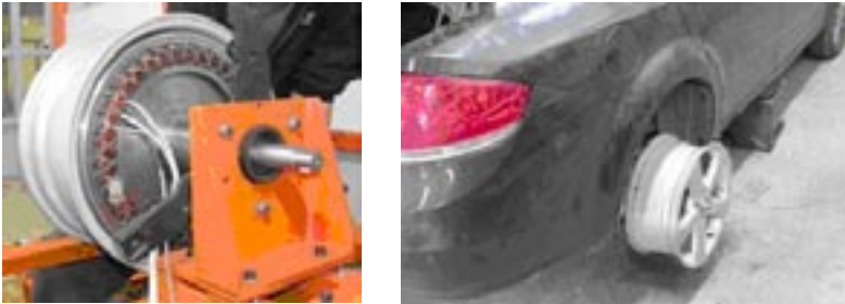
Fig. 23.5 Views of the Mekatro brushless DC machine before and after it was mounted on a vehicle. (Photos supplied by TÜBİTAK MRC.)
