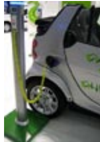
Fig. 19.12 ENEL charging post for electric vehicles. (Photo supplied by ENEA.)
