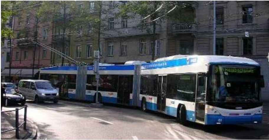
Fig. 12.3 25 metre long double articulated trolley bus in Zurich, Switzerland. (Photo: H. Schaffer.)
