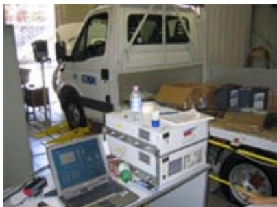
Fig. 19.2 IVECO Daily van on the ENEA roller bench during testing of hydrogen-methane fuel blends. (Photo supplied by ENEA.)
