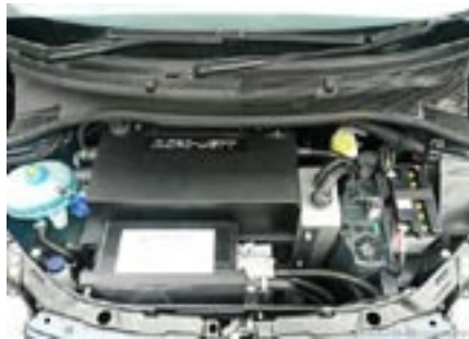
Fig. 19.11 Under the hood of the electric Fiat 500 prototype, modified by Micro-Vett. (Photo supplied by ENEA.)
