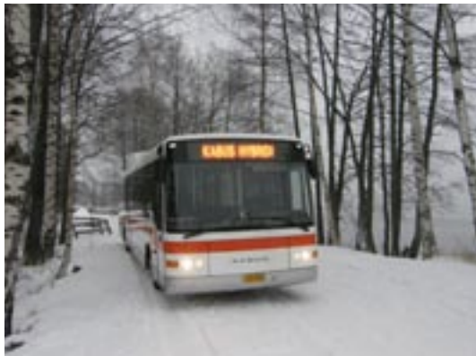
Fig. 17.3 Kabus launched a hybrid city bus in 2007. The bus has a lightweight full aluminium body and a parallel hybrid drive with supercapacitor energy buffer. It consumes 30% less fuel than a traditional city bus with similar capacity and performance. (Photo supplied by the Helsinki University of Technology.)
