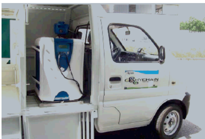
Fig. 19.10 VEM fuel cell hybrid utility van in the HY-CHAIN project. (Photo supplied by ENEA.)
