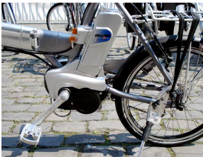
Fig. 8.2 Electric drive and battery of a Flyer foldable electric bicycle. (Photo: M. van Walwijk.)
