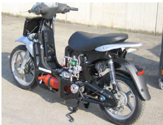
Fig. 19.9 Prototype fuel cell motorcycle with Arcotronics fuel cell. (Photo supplied by ENEA.)
