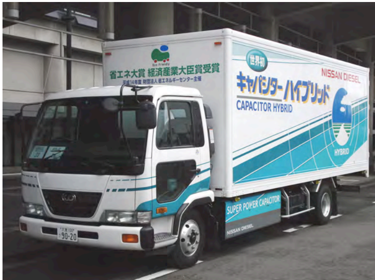
Fig. 9.2 Nissan hybrid truck with supercapacitors. (Photo: M. van Walwijk.)
