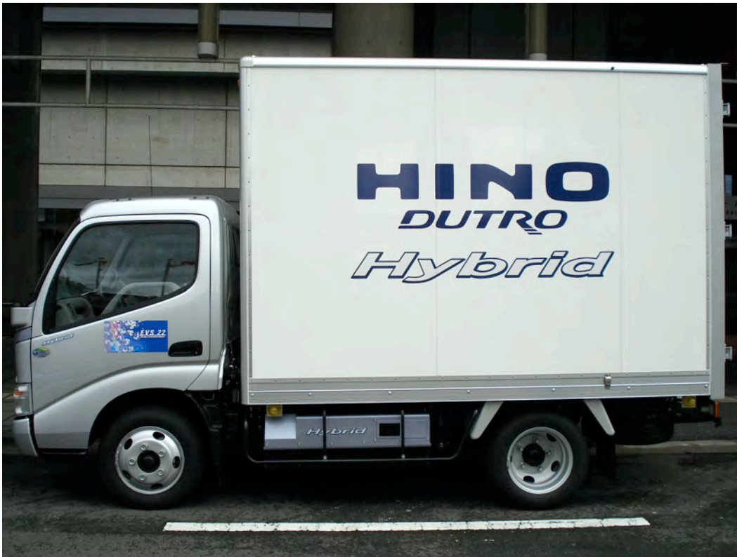
Fig. 22.5 Hino Dutro diesel electric hybrid distribution truck. (Photo: M. van Walwijk.)
