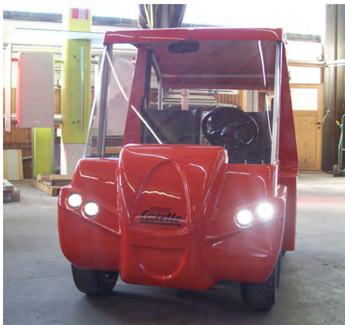
Fig. 13.3 Fuel cell powered vehicle, developed under the A3 'small traction' programme. (Photo courtesy ECHEM.)
