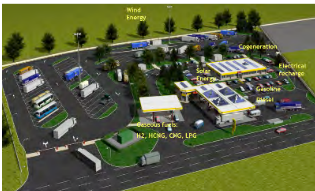
Fig. 16.6 AGIP MultiEnergy station at Collesalveti (Tuscany Region). (Picture supplied by ENEA.)
