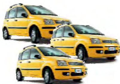
Fig. 16.4 Full-power fuel cell Fiat Panda and the fleet under realization for the Zero Regio project. (Photos supplied by ENEA.)
