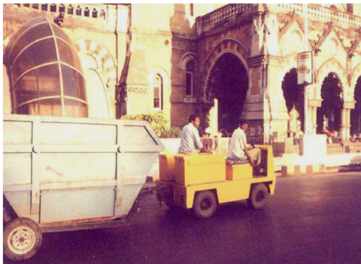
Fig. 21.3 Electric tow tractor used in vegetable waste collection, Mumbai, India. (Photo courtesy Clean Air Island, Mumbai, India.)
