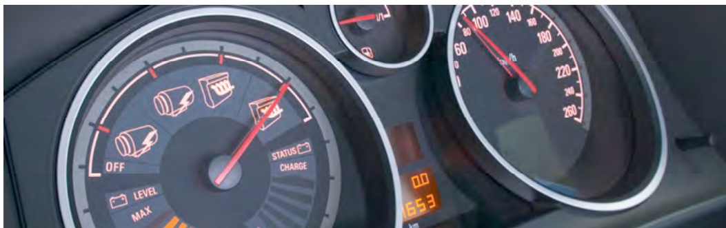
Fig. 17.1 Dashboard instrument indicating operation modes of a hybrid electric powertrain. (Photo courtesy PPS Automotive.)
