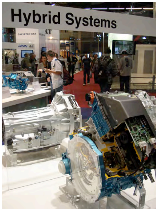
Fig. 4.1 Components for hybrid drives on display: gearboxes, electric motors and power electronics. (Photo: M. van Walwijk.)
