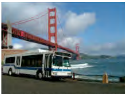
Fig. 8.1 40-foot BAE Systems-Orion diesel hybrid bus in San Francisco. (Photo courtesy BAE Systems ©.)
