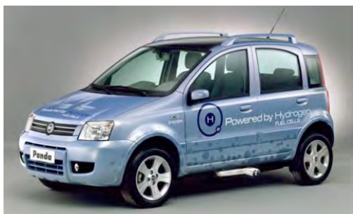
Fig. 16.4 Full-power fuel cell Fiat Panda and the fleet under realization for the Zero Regio project. (Photos supplied by ENEA.)
