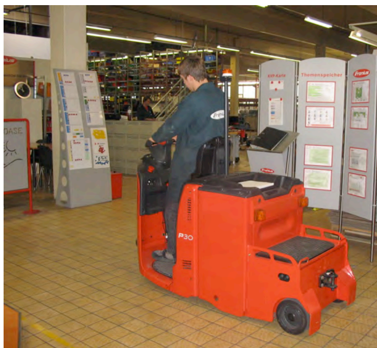
Fig. 13.2 Fuel cell powered forklift truck, developed under an A3 lighthouse project. (Photo courtesy Fronius International.)
