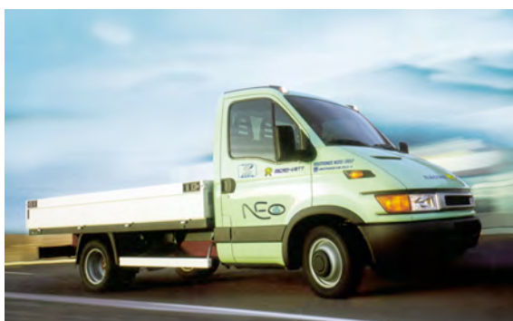
Fig. 16.8 NEO (No Emission Outfit) hybrid fuel cell commercial van. (Photo supplied by ENEA.)
