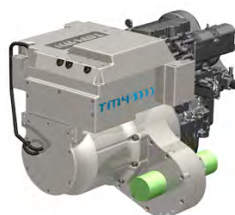
Fig. 15.2 TM4 motor/generator and Lombardini internal combustion engine for the hybrid version of the Cleanova. (Picture supplied by ADEME.)
