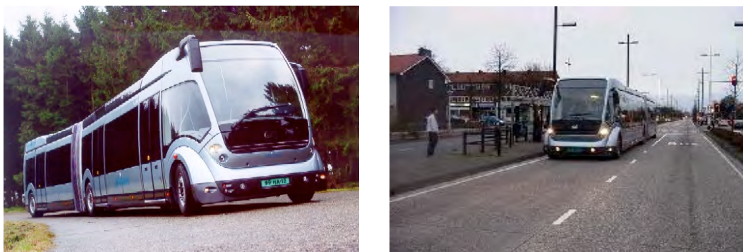
Fig. 17.2 The Phileas LPG electric hybrid bus on a test track (left) and in service (right). (Photos courtesy APTS-Phileas.)
