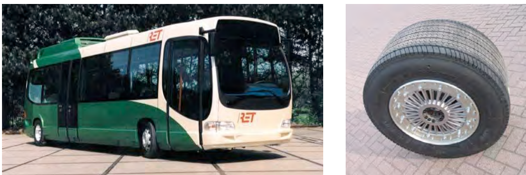
Fig. 17.4 Current (prototype) bus configuration and one of its drive wheels with electric wheel-hub motor TheWheel™. (Photos courtesy e-Traction®.)
