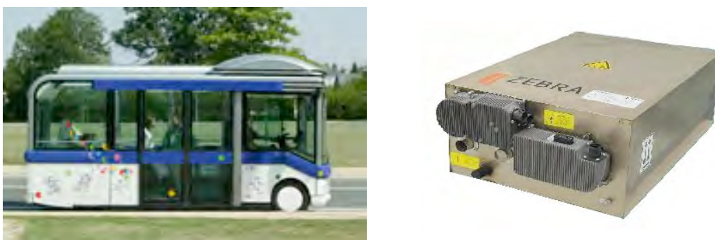
Fig. 15.4 View of the Microbus -note the very low and flat floor- and the ZEBRA battery block. (Photos supplied by ADEME.)
