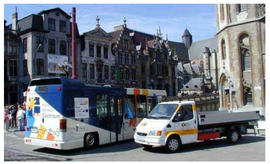
Fig. 10.1 Hybrid bus of the city of Luxemburg and Vito hybrid van (HEVAN project), here pictured in Ghent, Belgium. (Photo supplied by Vito.)
