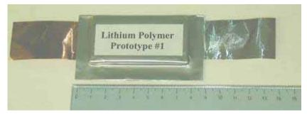
Fig. 13.1 ENEA Lithium metal softpack (710 mAh – 167 Wh/kg) prototype for EV applications. (Photo supplied by ENEA.)
